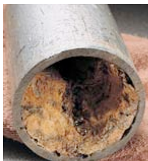
cross sections of pipes showing extensive calcium carbonate deposition
