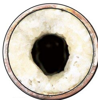
cross sections of pipes showing extensive calcium carbonate deposition
